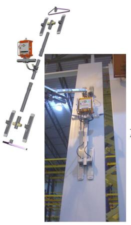
Using 4 x 440 lbs double suction pads, the lift capacity of the unit can be increased to 1760 lbs in defined configurations.
