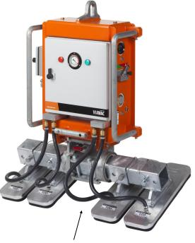
Using 4 x 220 lbs suction pads, the unit can be configured for both horizontal and vertical wall panels weighing up to 880 lbs.
